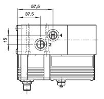
1 Valves are delivered with M4 x 50 mounting screws
